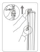
Raise the top hook using the coloured button to release the top locating pin.
